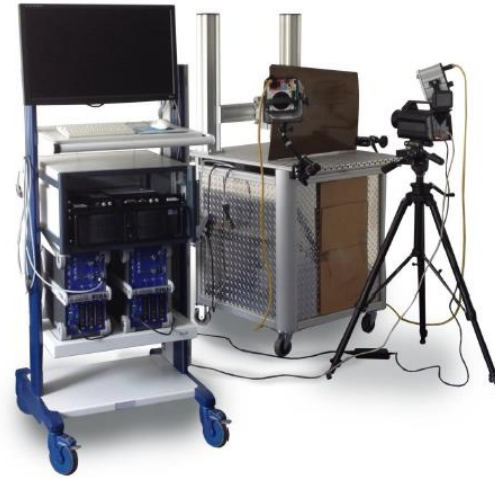
Thermography: Pulse, Transient, Lock-in
